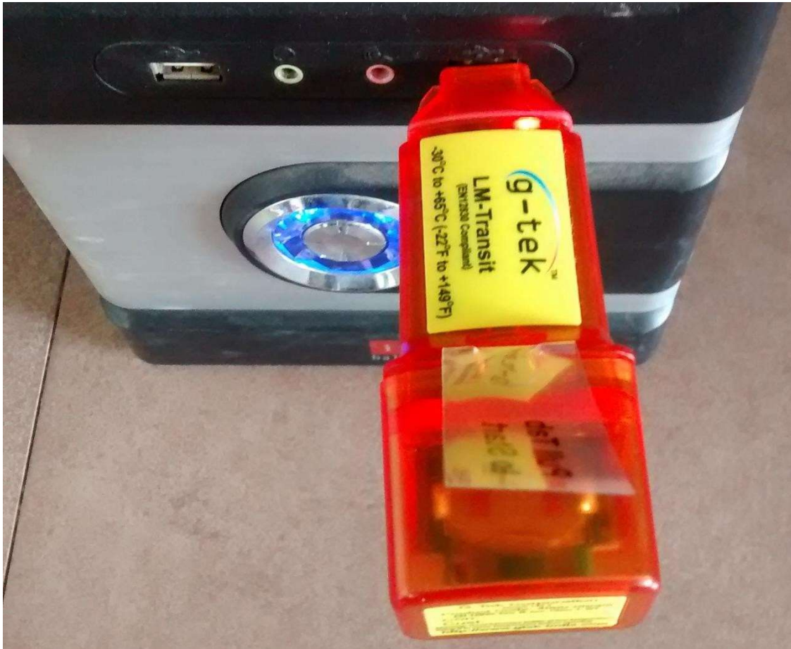
Figure 4 Connection of LM Transit to PC via USB port
