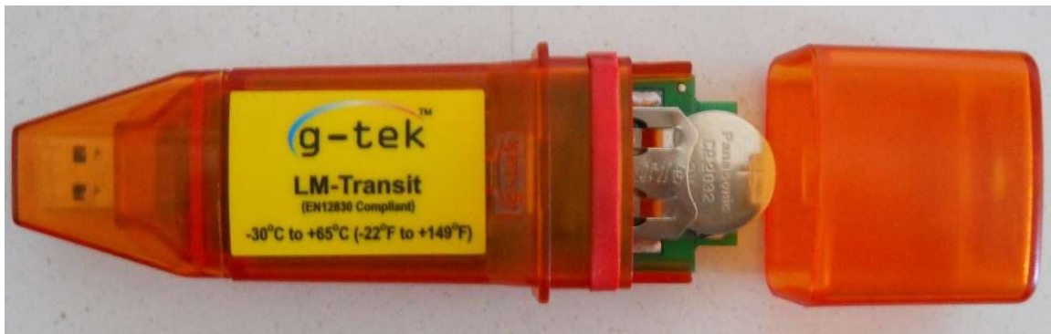
Figure 5 Open the Sensor cover to replace the Battery
